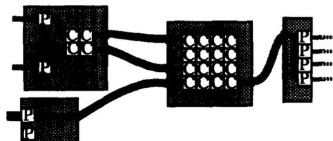
**Figure 1** One single system composed of compute memories, C, and port memories, P.
