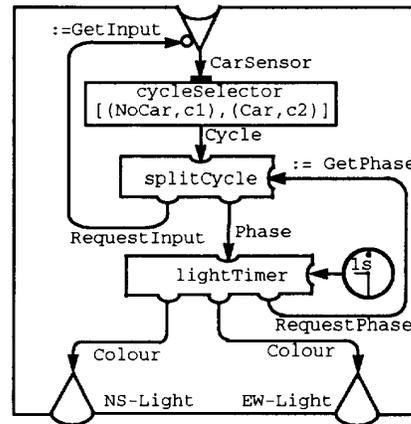
Figure 7 The content of `trafficControl`. The definition is partly in the graphical  $H_{US}$  language and partly in the purely functional  $H_{UF}$ .
