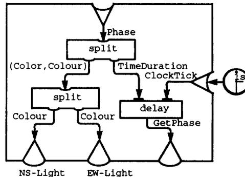
Figure 10 Definition of the box lightTimer.
